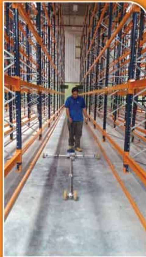
SUPERFLAT FLOOR SURVEY
