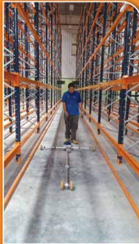
SUPERFLAT FLOOR SURVEY
