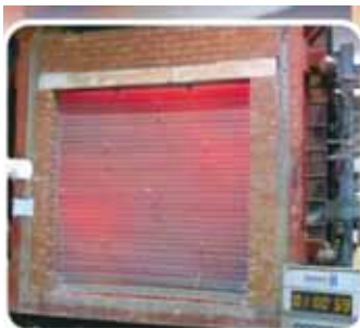
AFTER 1 hr FIRE TESTING
