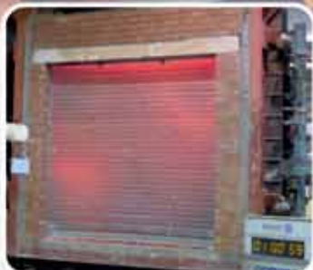
AFTER 1 hr FIRE TESTING
