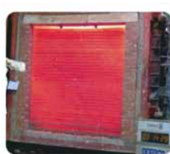
AFTER 3 hrs FIRE TESTING
