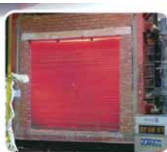
AFTER 2 hrs FIRE TESTING
